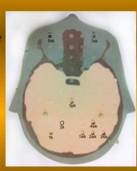
TLD located in phantom scan and shown on treatment plans
