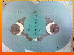
TLD located in phantom scan and shown on treatment plans
